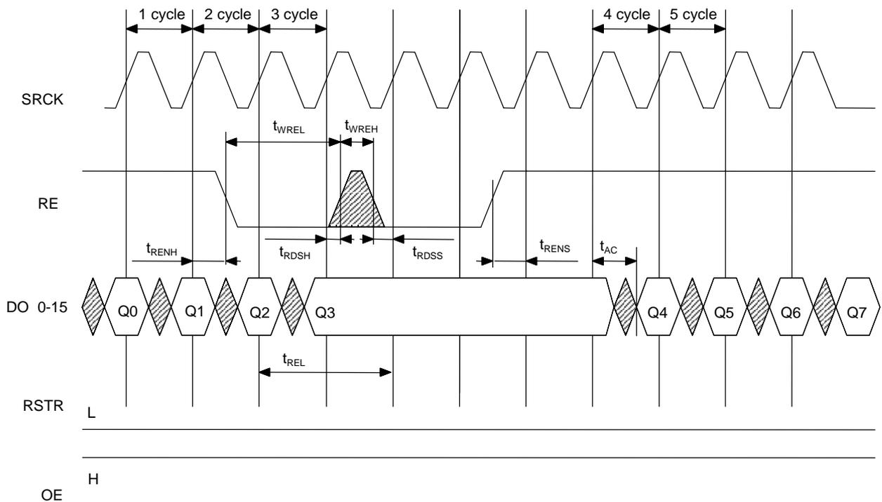
**Read Cycle Timing (Output Enable)**
