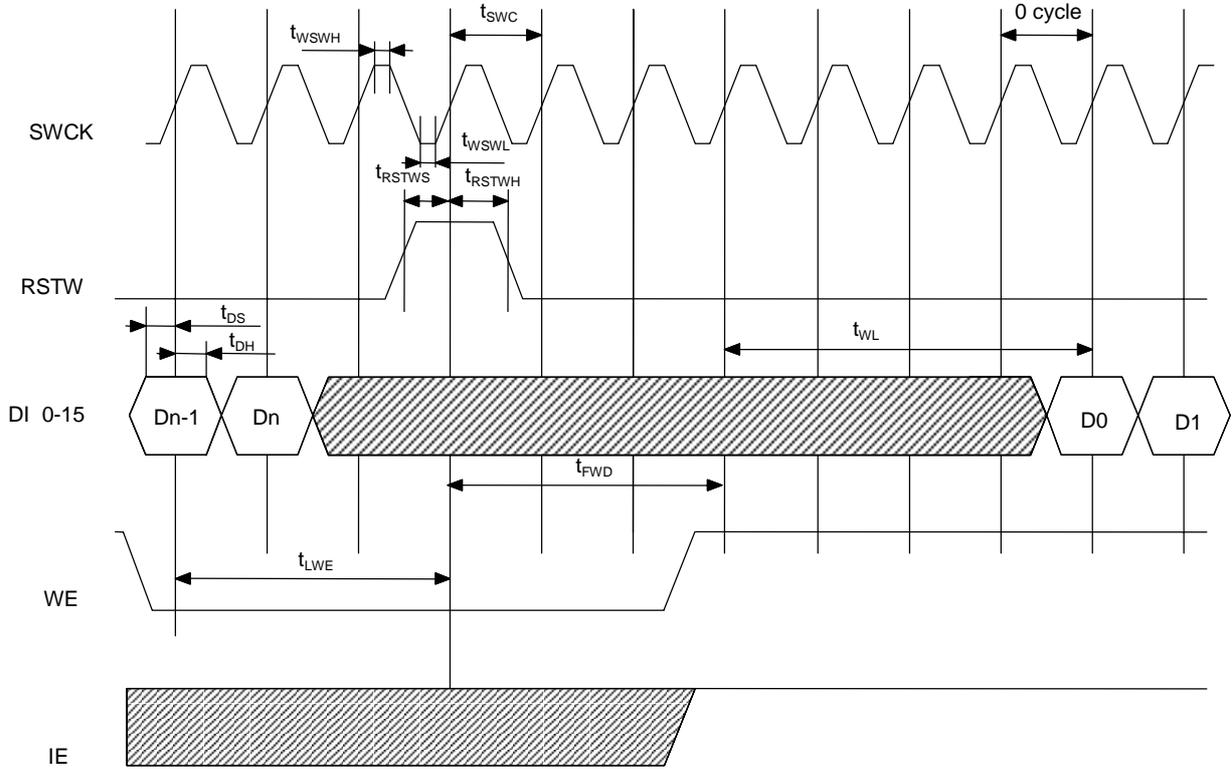
\*After write reset, WE should be remained high for 2 cycles after driving WE high first.
