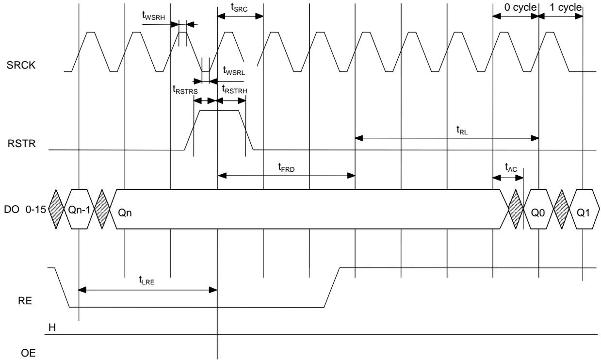
\*After write reset, RE should be remained high for 2 cycles after driving RE high first.
