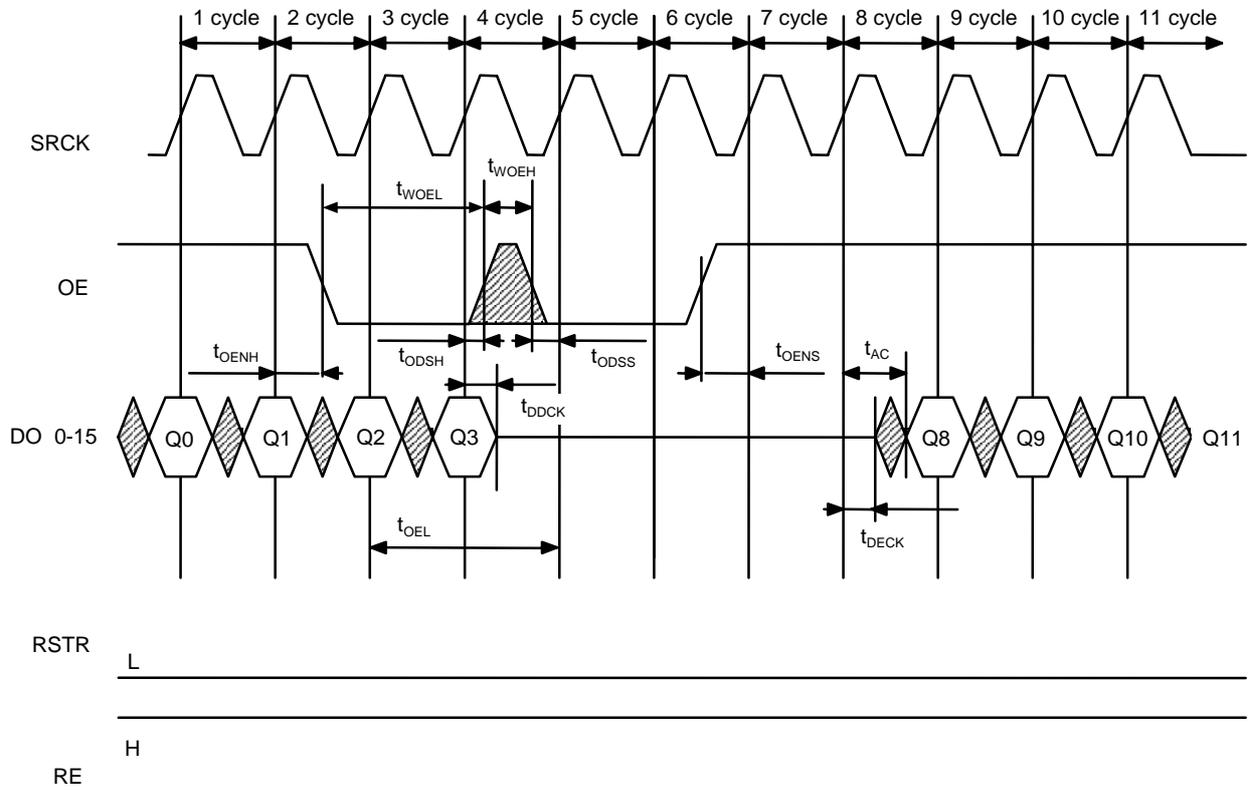
**Read/Write Cycle Timing (New Data Read)**
