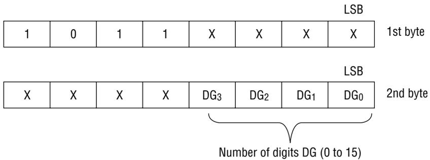
The relation between the value of DG to be set and COM under display control is as follows:
