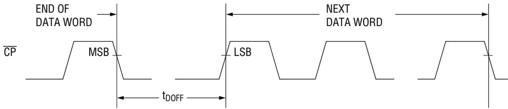
DATA INPUT OFF TIME  $t_{DOFF} = 32T_{min}$  ( $T=1/f_{osc}$ )
