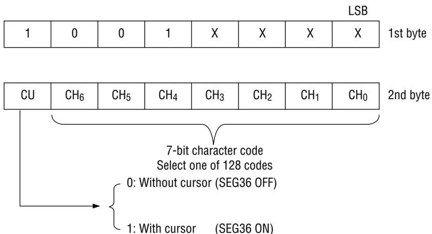
An automatic address increment function is built in. To write multidigit display character codes, issue the Address Set command. To transfer the second and later digit display character codes, the first byte (operation code) of the Character Code command is not required. Input the second byte.
