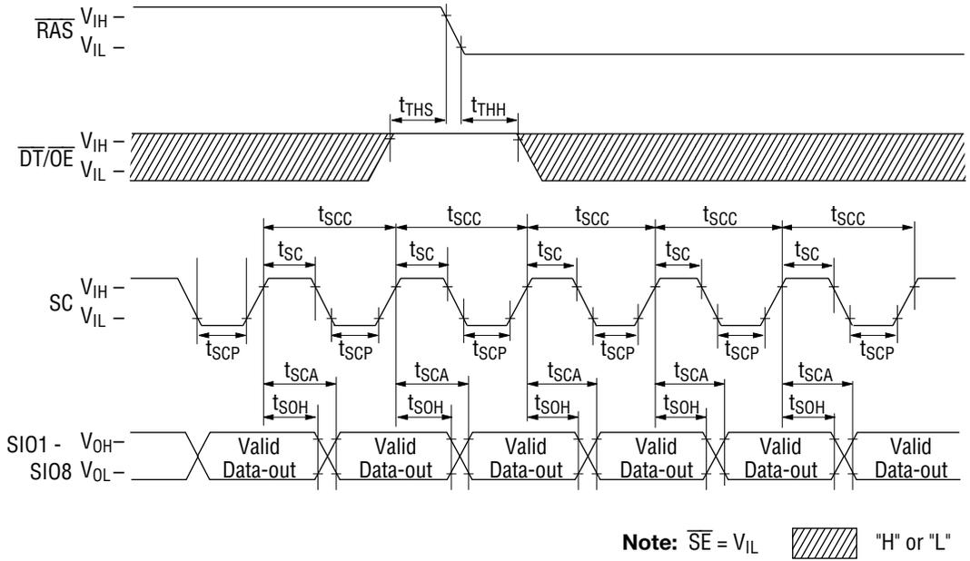
**Serial Read Cycle ( $\overline{SE}$  Controlled Outputs)**
