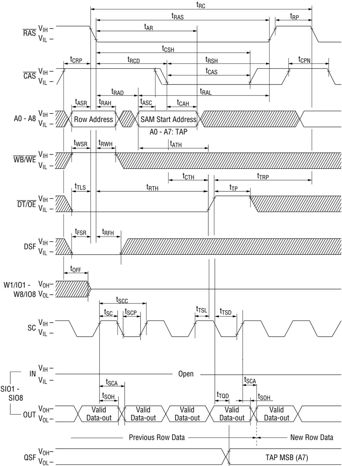
Note:  $\overline{SE} = V_{IL}$  "H" or "L"
