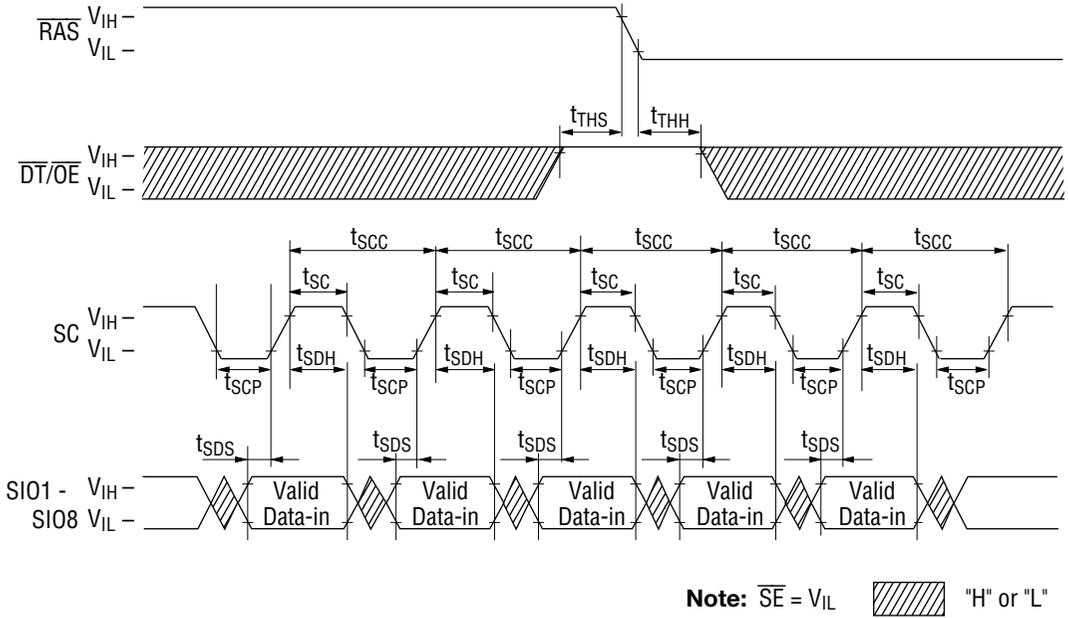
**Serial Write Cycle ( $\overline{SE}$  Controlled Inputs)**
