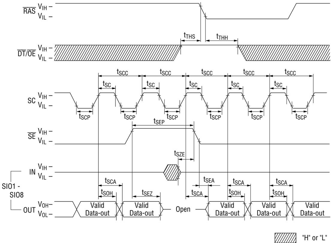
**Serial Write Cycle ( $\overline{SE} = V_{IL}$ )**
