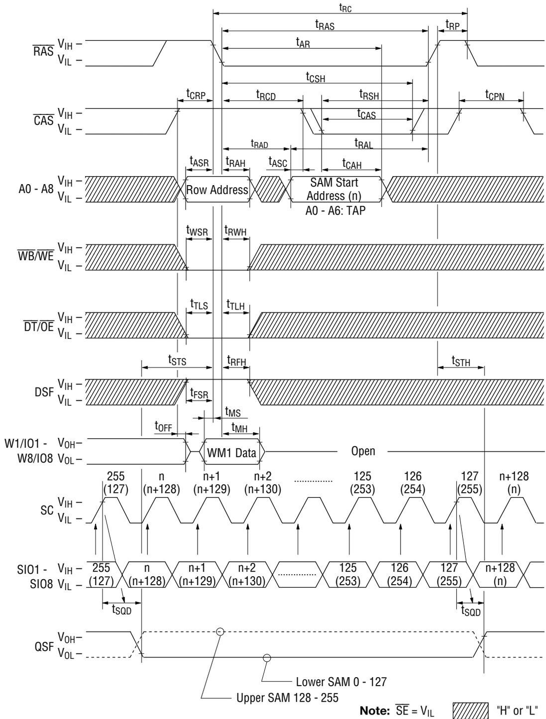
**Serial Read Cycle ( $\overline{SE} = V_{IL}$ )**
