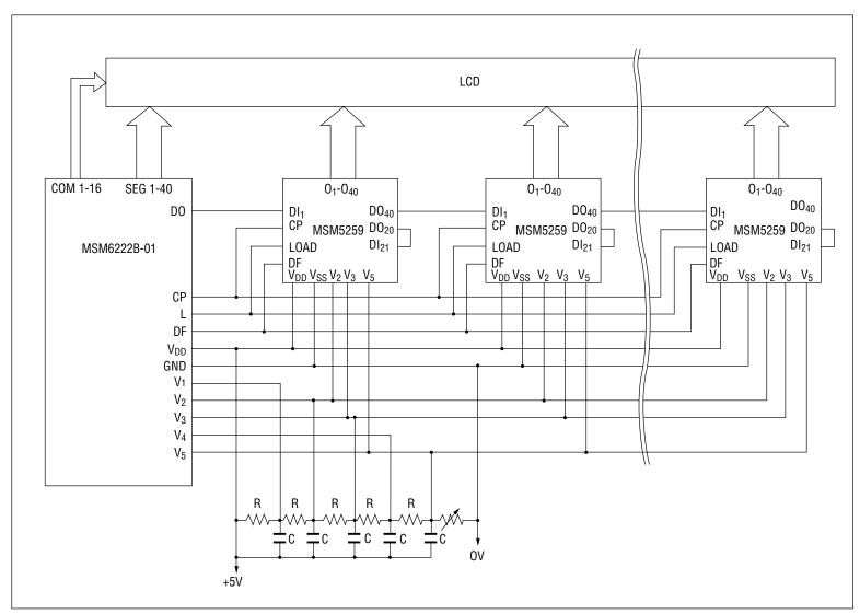
The MSM5259 is applicable to a static LCD by setting  $V_2$  and  $V_5$  at ground level, connecting  $V_3$  to  $V_{DD}$  and inputting COMMON SIGNAL to DF pin.
