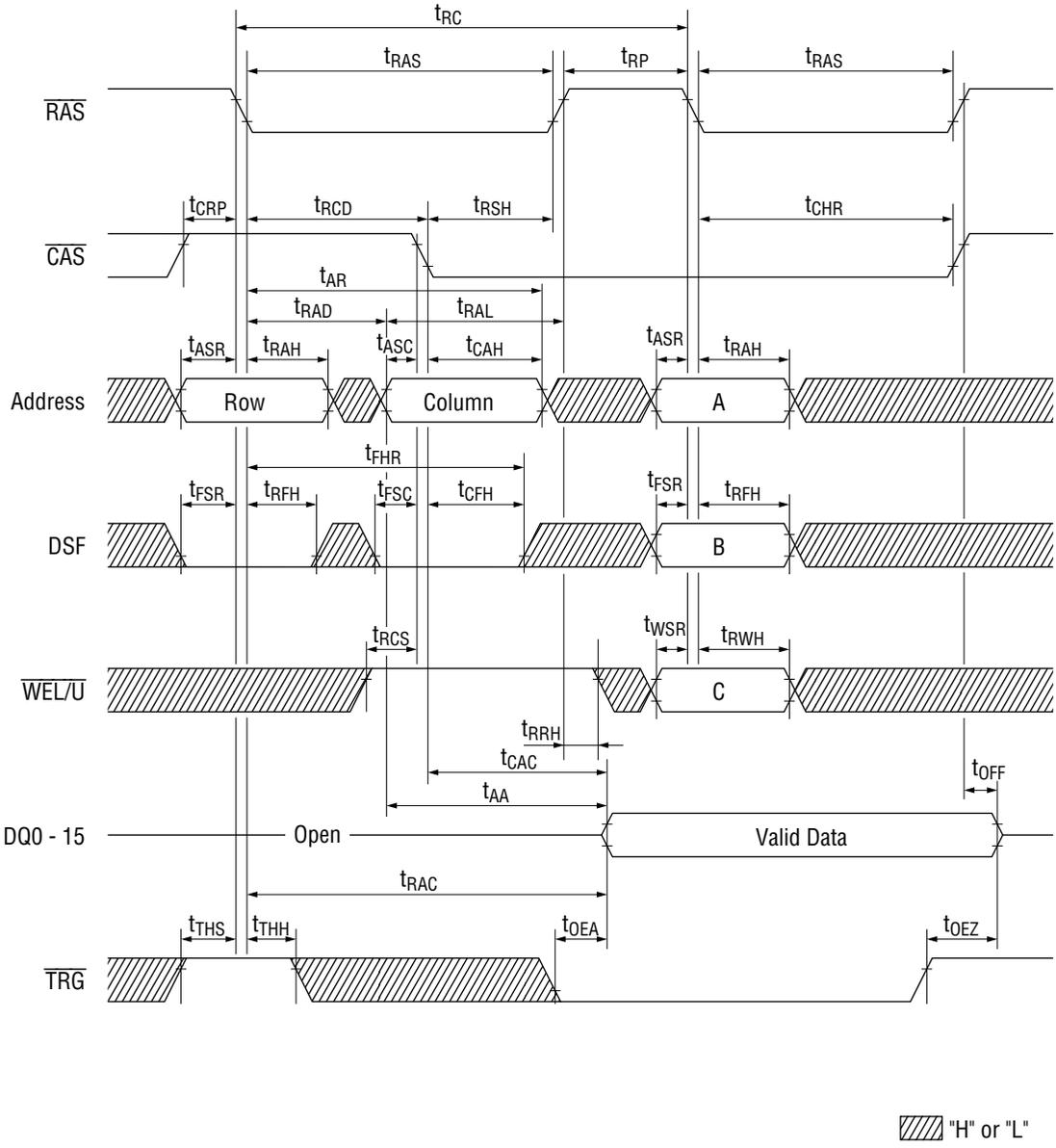
**Note:** The type of CBR operations are determined by the logic states of "A", "B" and "C".
