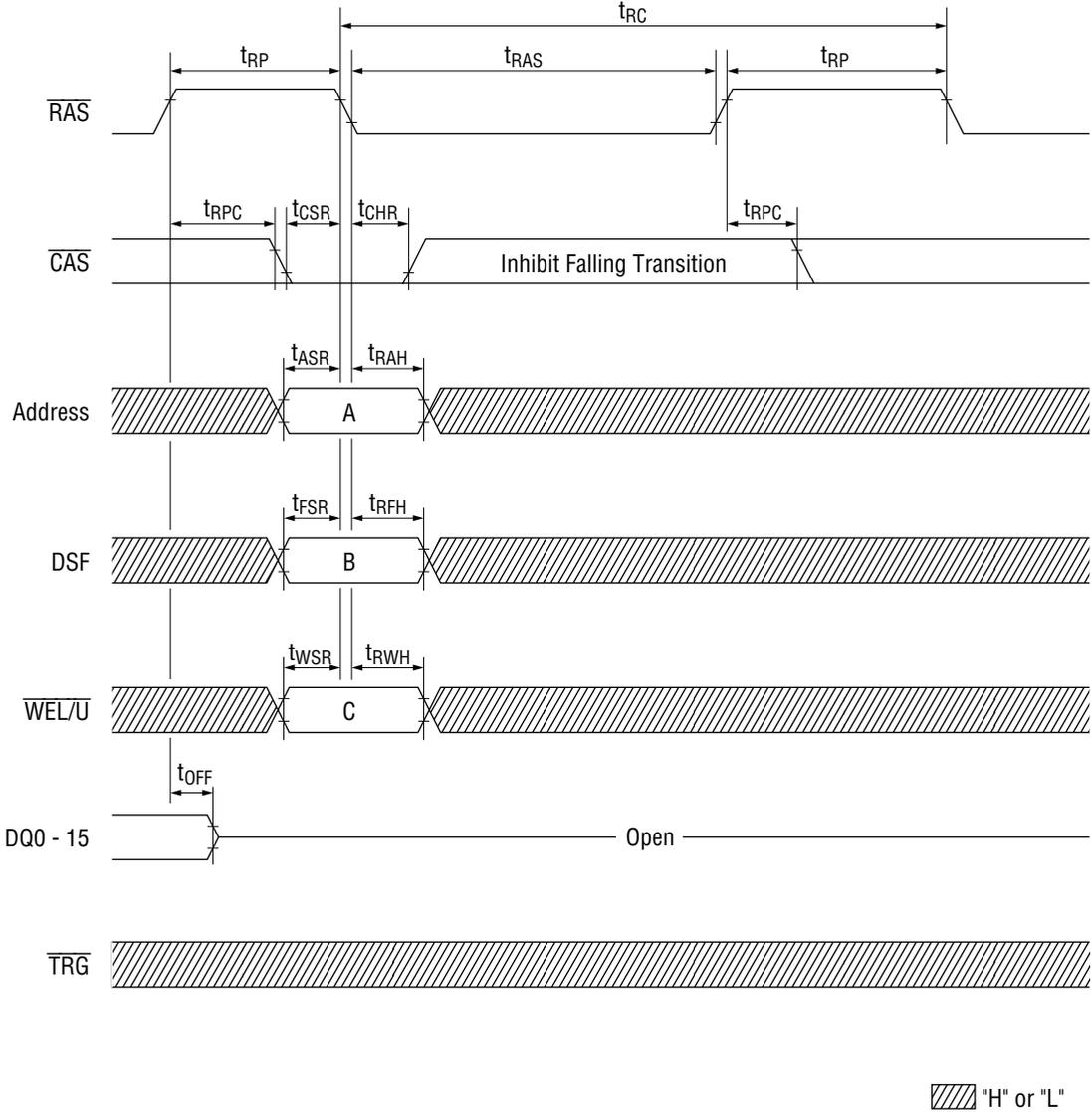
**Note:** The type of CBR operations are determined by the logic states of "A", "B" and "C".
