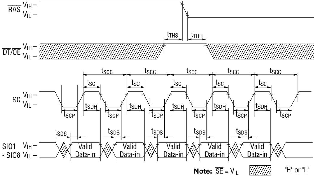
**Serial Write Cycle ( $\overline{SE}$  Controlled Inputs)**
