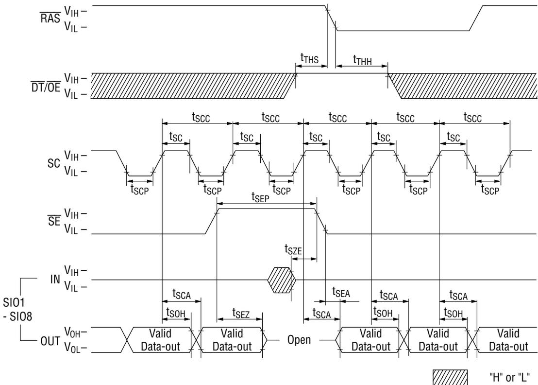
**Serial Write Cycle ( $\overline{SE} = V_{IL}$ )**
