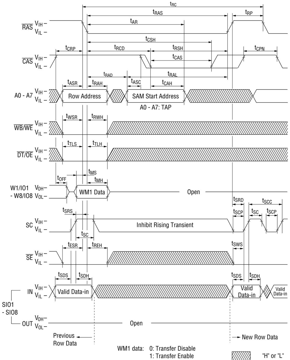
**Serial Read Cycle ( $\overline{SE} = V_{IL}$ )**
