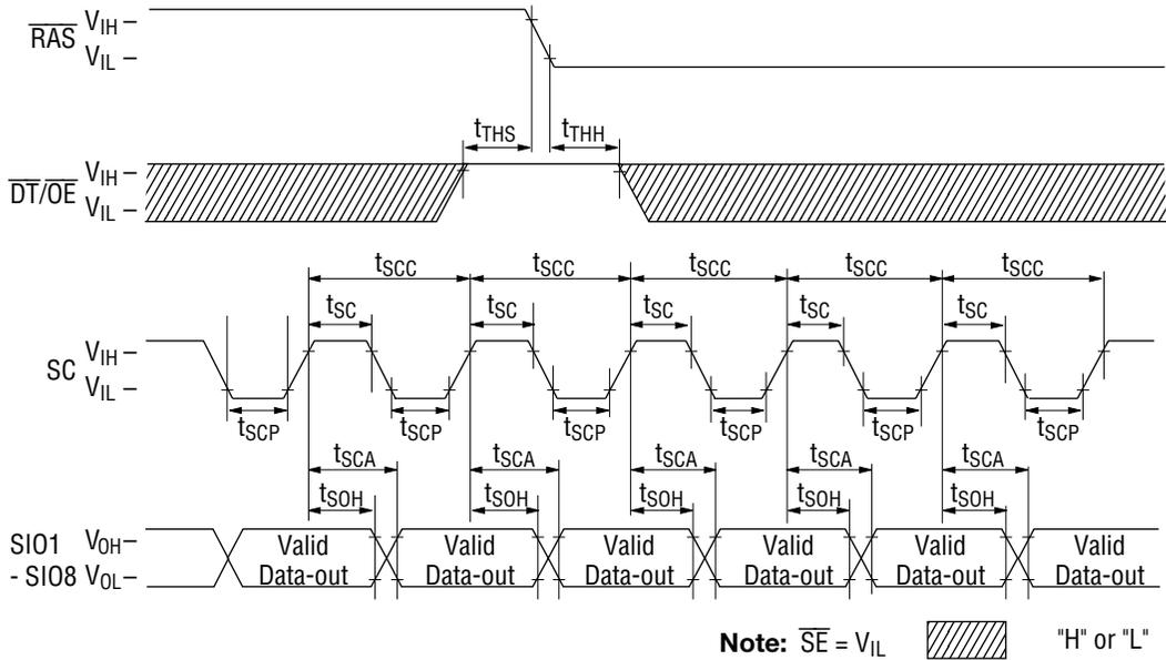
**Serial Read Cycle ( $\overline{SE}$  Controlled Outputs)**
