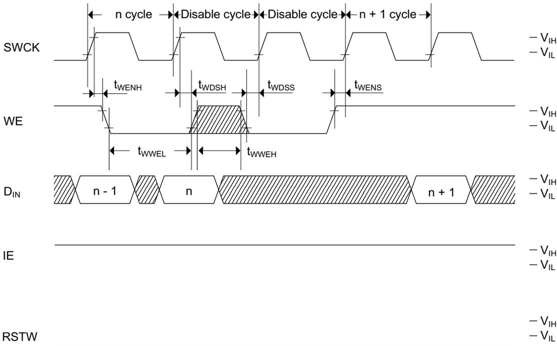
Write Cycle Timing (Input Enable)
