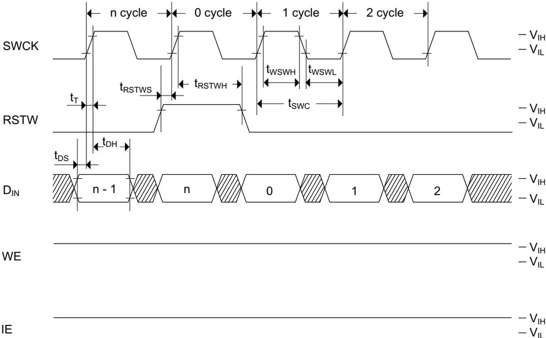
**Write Cycle Timing (Write Enable)**
