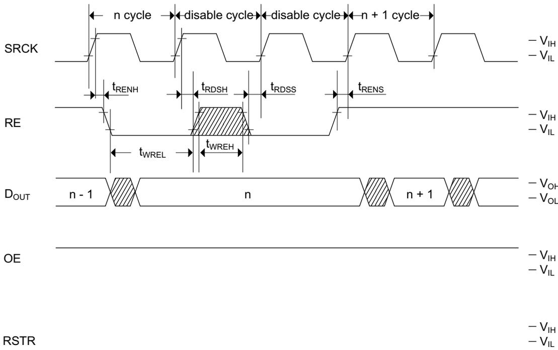
Read Cycle Timing (Output Enable)
