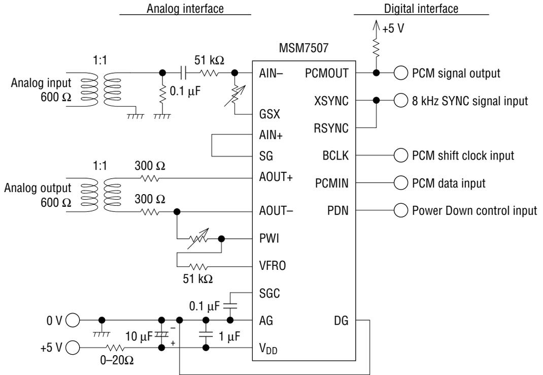
**FREQUENCY CHARACTERISTICS ADJUSTMENT CIRCUIT**
