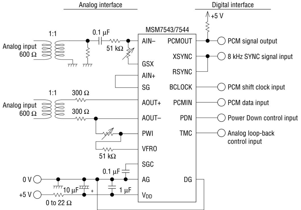
**FREQUENCY CHARACTERISTICS ADJUSTMENT CIRCUIT**
