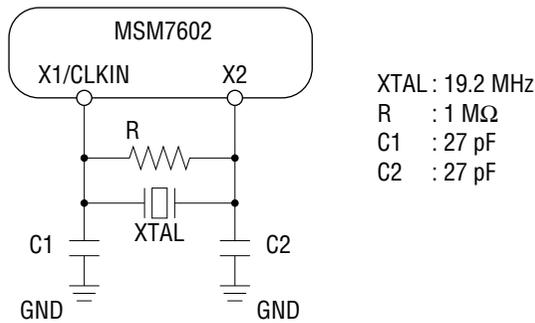
**External Clock Input Circuit Example**
