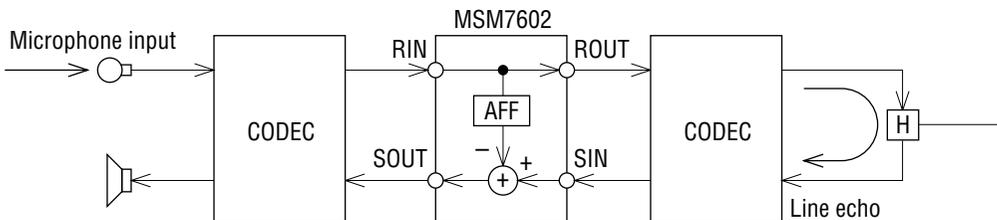
Example 3: Canceling line echo in a cascade connection (to handle line echo from microphone input)
