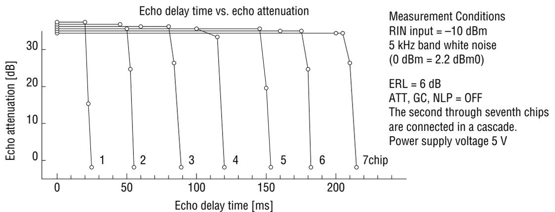
Note: The characteristics above are for the MSM7543 ( $V_{DD}$  5 V,  $\mu$ -law interface). The MSM7566 ( $V_{DD}$  3 V,  $\mu$ -law interface) provides the same characteristics without input and output levels. Refer to are PCM CODEC data sheet.
