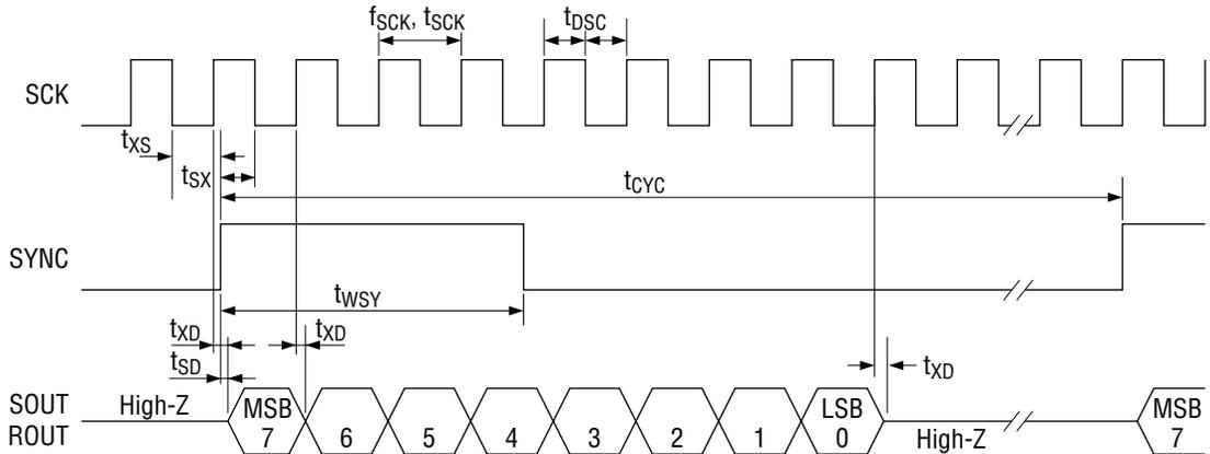
**Serial Data Output Timing (Serial Mode)**
