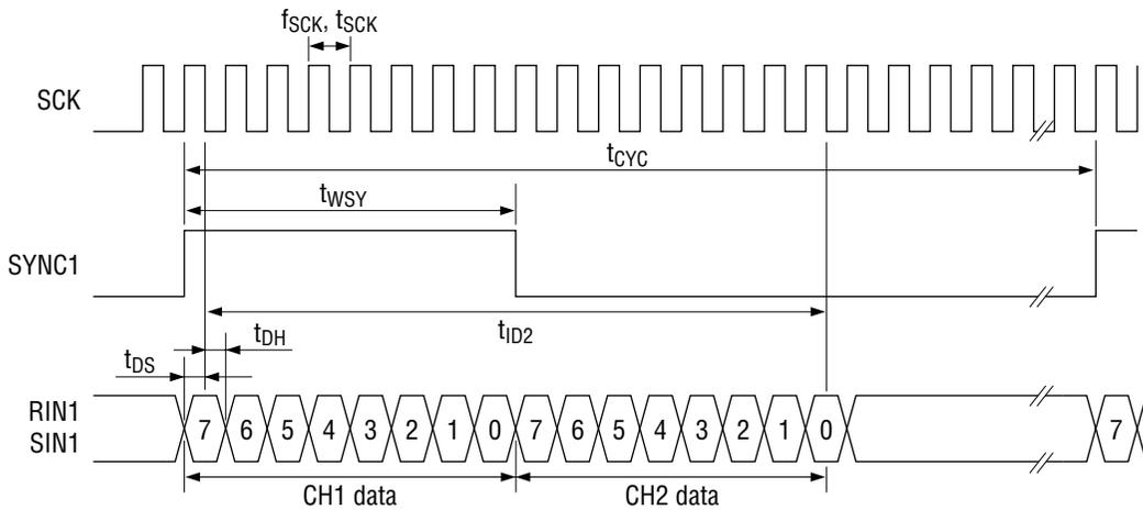
**Serial Data Output Timing (Parallel Mode, FTF Mode)**
