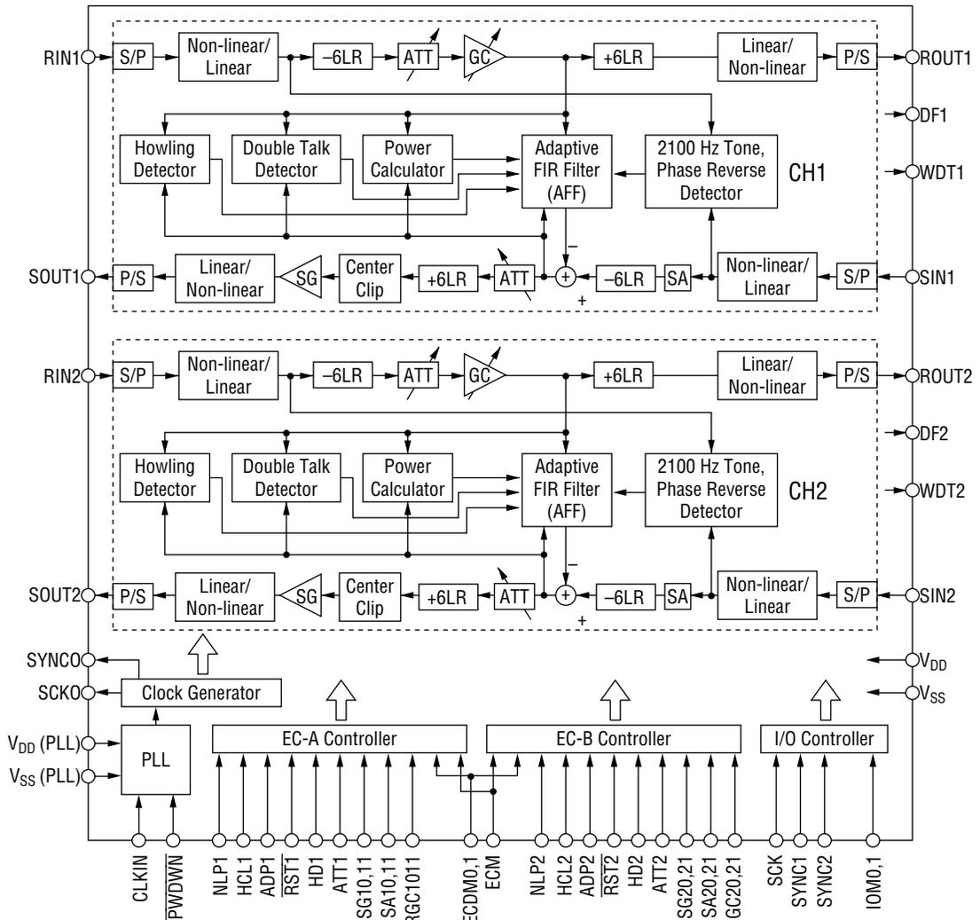
The above diagram shows internal connections for 2-channel parallel mode. The internal connections for 2-channel serial I/O mode and 1-channel cross-connected mode are shown below.
