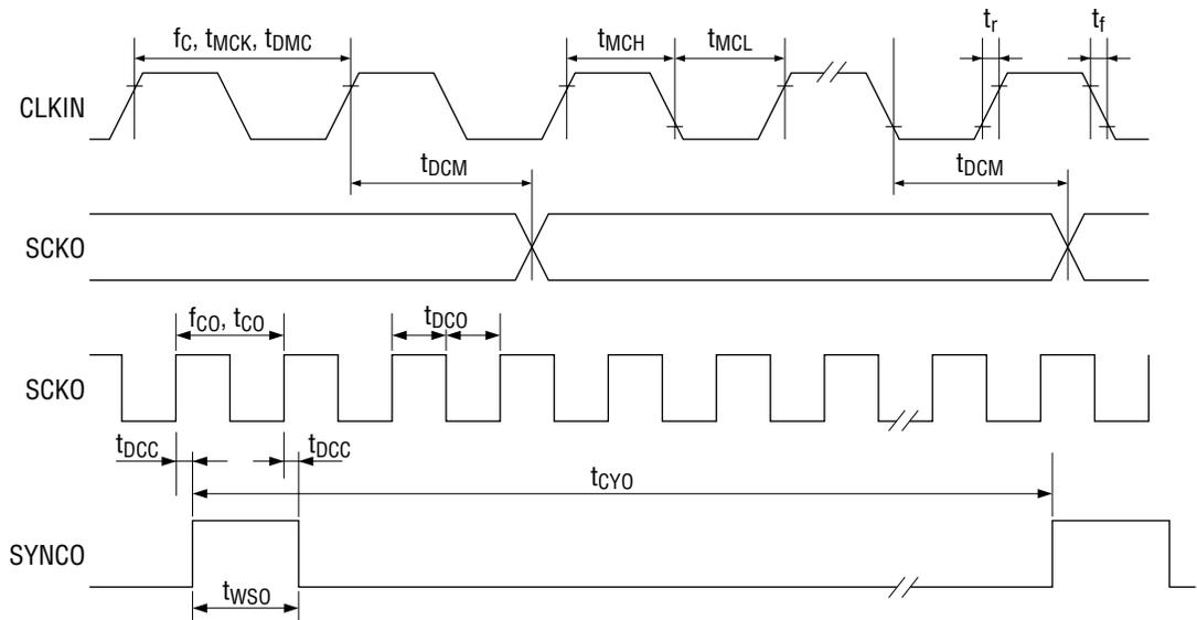
**Serial Data Input Timing (Parallel Mode, FTF Mode)**
