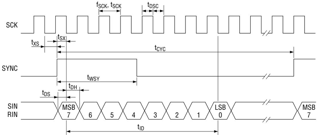
**Serial Data Input Timing (Serial Mode)**
