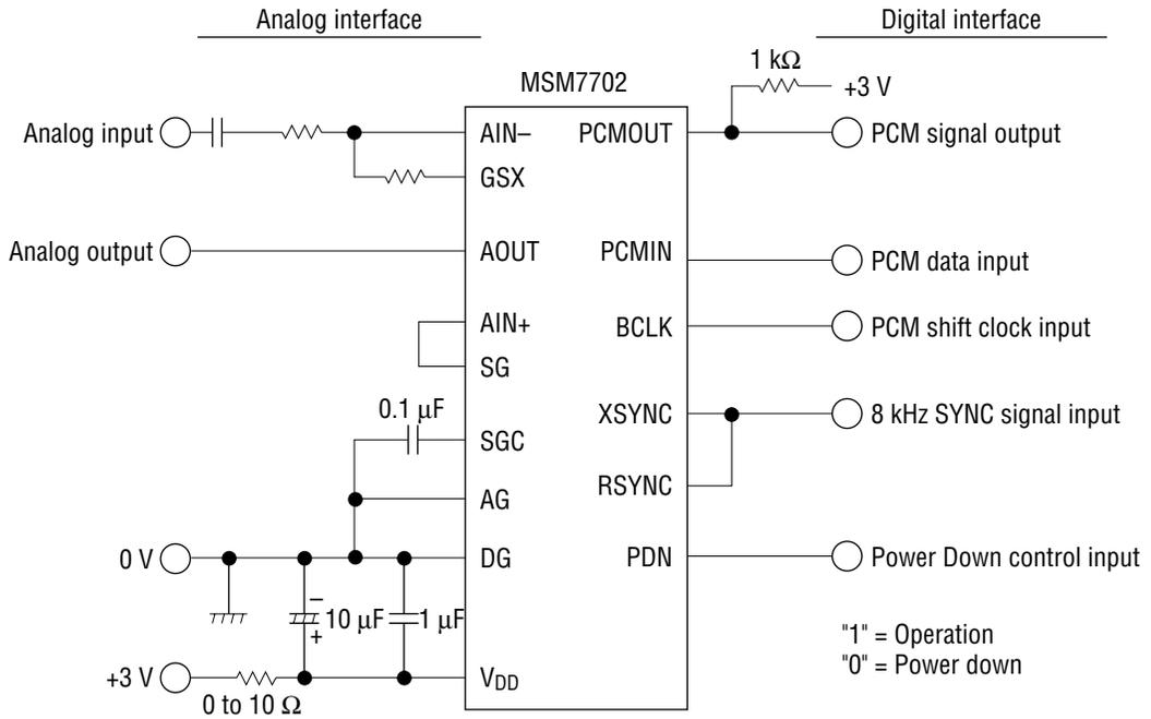
The analog output signal has a maximum amplitude of ±1.0 V above and below the offset voltage level of  $V_{DD}/2$ .
