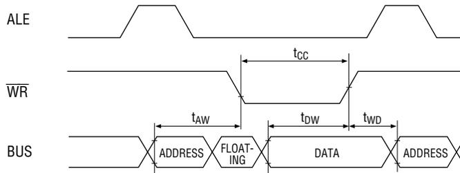
**Low-order 4 bits input/output of port 2 when expanded I/O port is used (in external program memory access mode)**
