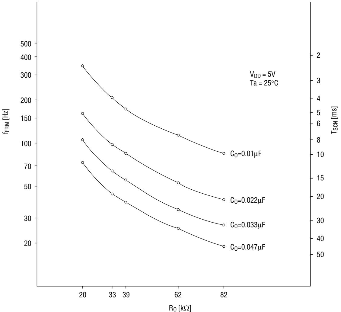
f<sub>FRM</sub> and T<sub>SCN</sub> vs. R<sub>0</sub> vs. C<sub>0</sub>
