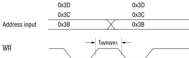
Figure 4.5 When 0x3B to 0x3D are continuously written at the same address (This is a rare case)
