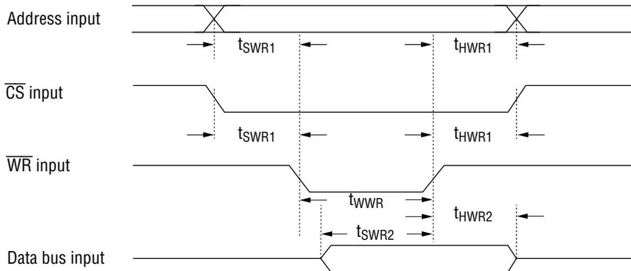
Figure 4.1 Write Timing
