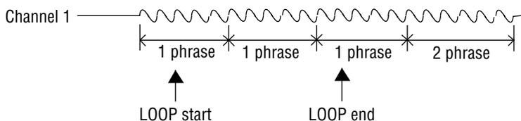
**Figure 9-2 LOOP Command Execution Example**
