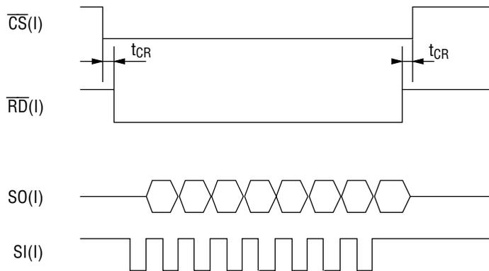
**Command input timing in parallel input interface**
