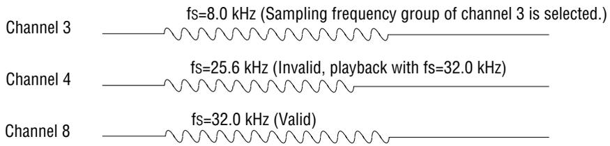
**Figure 3.3 When channel 3, 4 and 8 are played back simultaneously.**
