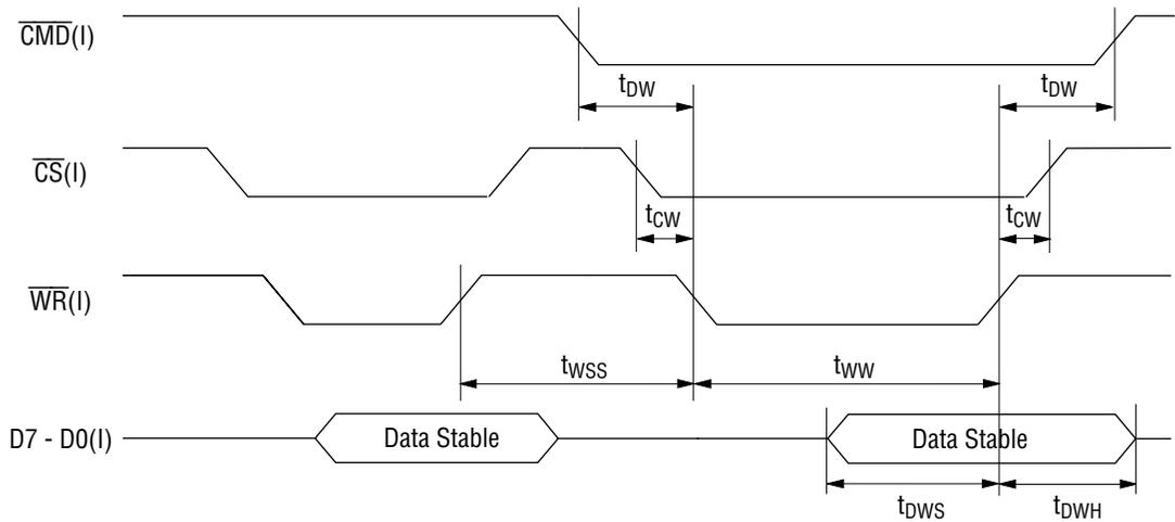
**Data Write Timing, Serial Input**
