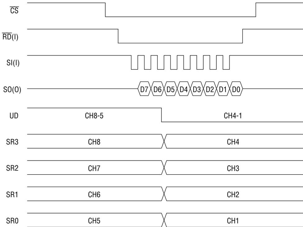
**Figure 8-2 Read timing in serial input interface**
