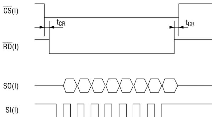
Figure 7-4 Serial input read cycle timing
