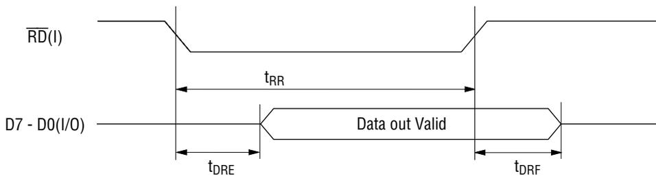
**Figure 8-1 Read timing in parallel input interface**
