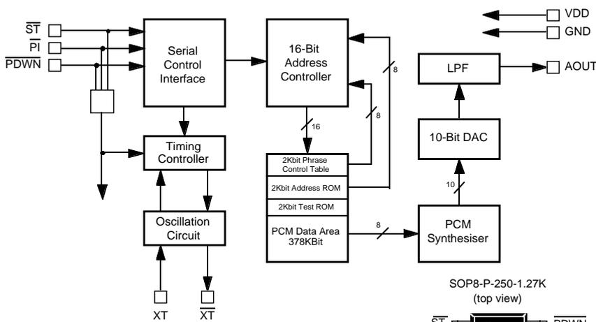
FIGURE 2. Block diagram and pin assignment
