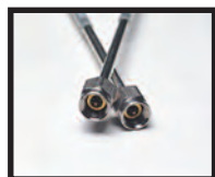
K101M-R ④⑥ K Male In-Line Cable Connector, DC-40 GHz for 3 mm cable K101M-085-R ④ for 2.16 mm cable
