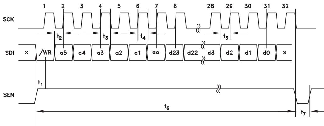
Figure 29. Serial Port Timing Diagram - WRITE
