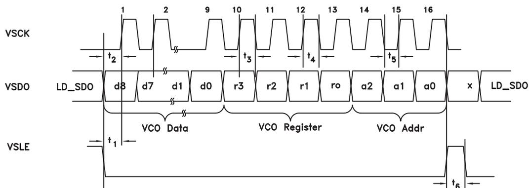
Figure 31. VCO Serial Port Timing Diagram - WRITE ONLY
