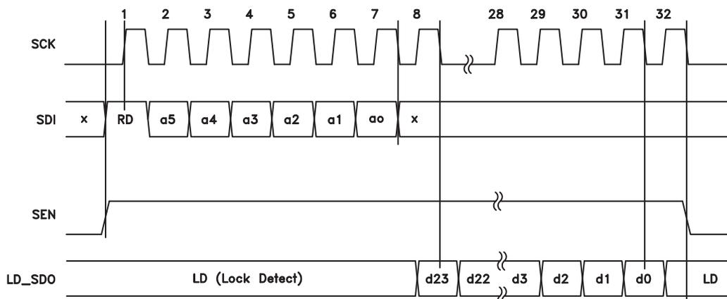
Figure 30. Serial Port Timing Diagram - READ
