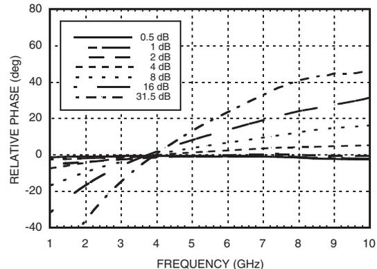
**0.5 dB LSB GaAs MMIC 6-BIT DIGITAL POSITIVE CONTROL ATTENUATOR, 2.4 - 8.0 GHz**
