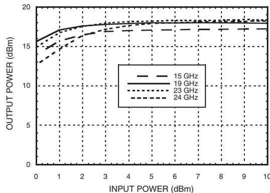
**GaAs MMIC x2 ACTIVE FREQUENCY MULTIPLIER, 13 - 24.6 GHz OUTPUT**
