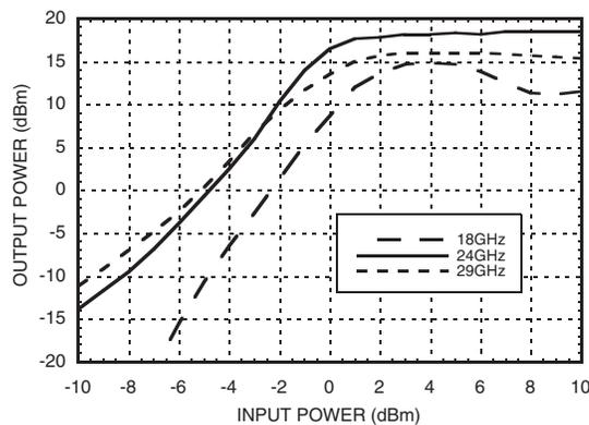
**GaAs MMIC x2 ACTIVE FREQUENCY MULTIPLIER, 18 - 29 GHz OUTPUT**
