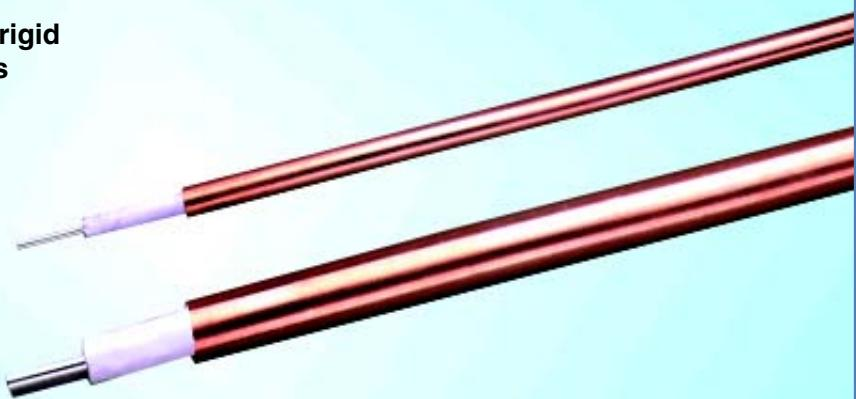
**Coppersol-CLL** employs a thin tubular copper outer conductor and low-density PTFE dielectric which provide the lowest loss and highest shielding giving it significant performance advantages over semirigid coax of similar size.
