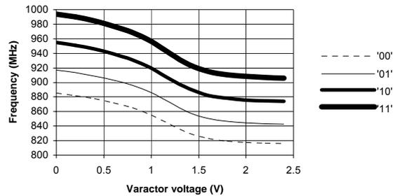
**Figure 7. RF Frequency vs. Varactor Voltage and VCO Frequency bit (V<sub>DD</sub> = 2.25V)**
