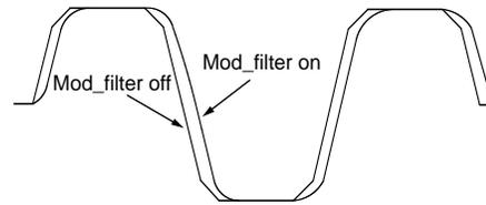
Figure 23. Modulator Waveform with and without Filtering
