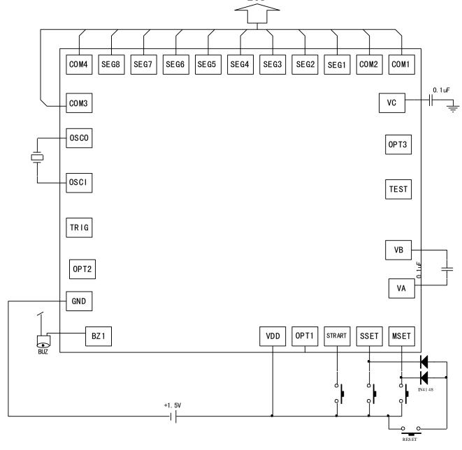
NOTE: The chip substrate must be floated or connected to VDD.
