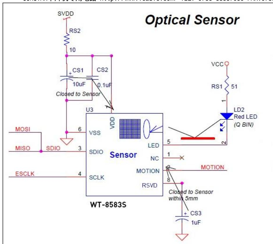
Figure 8. Sensor Circuitry
