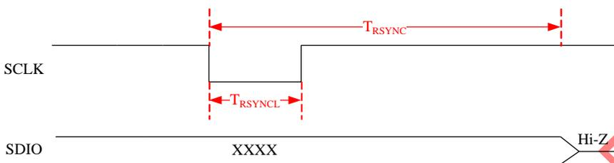
Figure 12. Re-synchronization Operation
