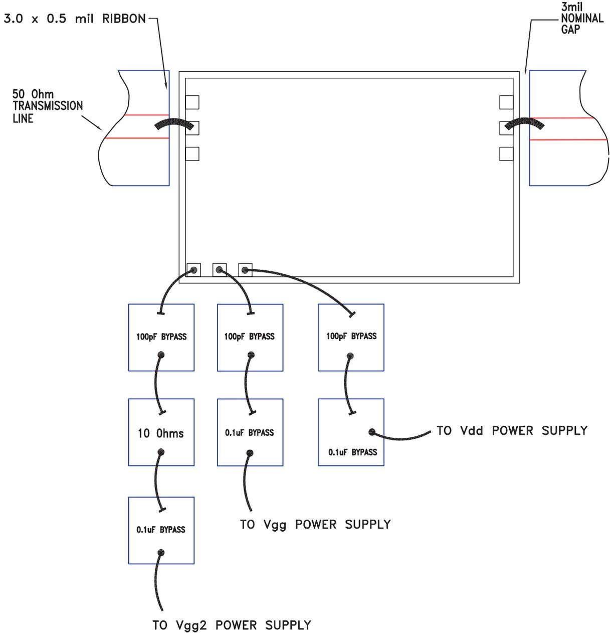
Note 1: Bypass caps should be 100 pF (approximately) ceramic (single-layer) placed no farther than 30 mils from the amplifier.
