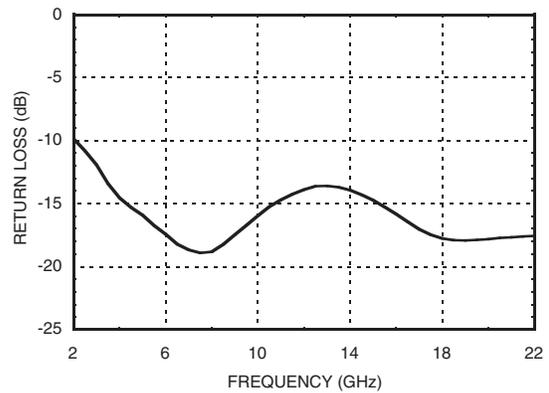
Note: Measured Performance Characteristics (Typical Performance at 25°C) Vd= 2.0 V, Id = 55 mA
