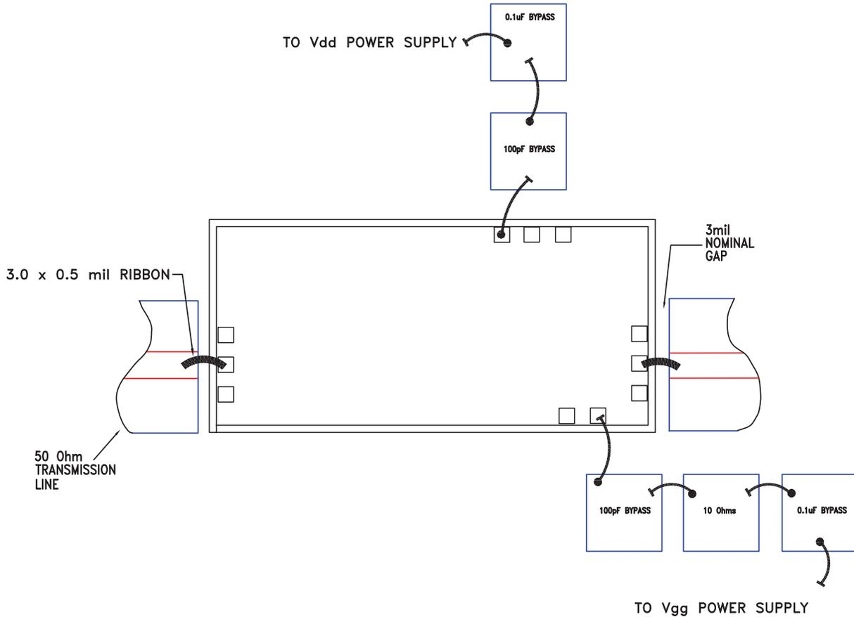
Note 1: Bypass caps should be 100 pF (approximately) ceramic (single-layer) placed no farther than 30 mils from the amplifier
