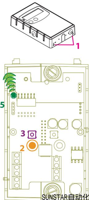
1. Back out set screws along bottom edge of enclosure cover and remove cover.
