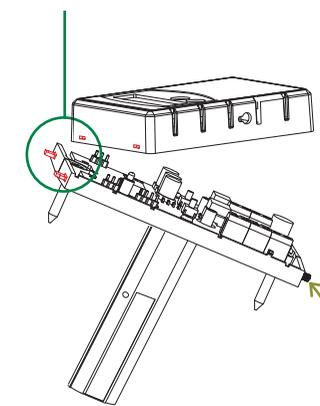
Once lid closed, insert set-screws to lock enclosure. Requires 1/16" Allen Wrench
