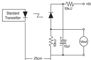
**Test Condition of Transmission Distance**
