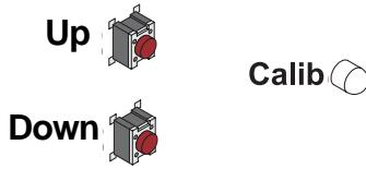
**3. PUSHBUTTON Up and Down:** Pressing one of the two buttons will adjust the measuring value in steps of 0.1% up or down to the reference value. The actual measuring value can be measured with the analogue output.
