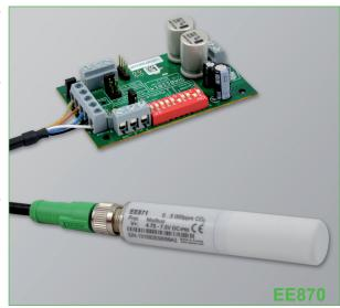
The measured data range of up to 10,000ppm is available on the analog outputs. Several voltage and current ranges can be selected with jumpers. Additionally, the data is available on the Modbus RTU interface, which can be configured by the user with DIP switches on the board.
