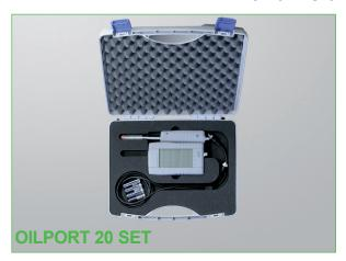
The carrying cases can accommodate the measuring equipment with optional calibration devices. The accuracies of the measured values are traceable to international standards, administrated by NIST, PTB, BEV...
