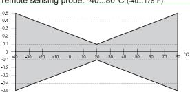
Temperature dependence of electronics  $typ. \pm 0.007^{\circ}C/^{\circ}C$ Response time  $t_{ss}$ : typ. < 6min
