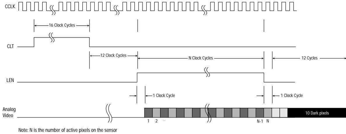
**Figure 4: Slave Mode Timing Diagram**
