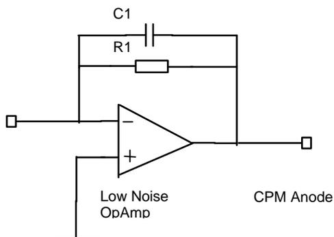
Fig. :6 Preamplifier for DC Mode (I/U conversion) (Proposal)
