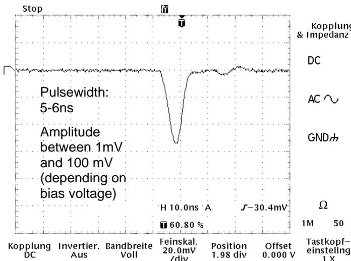
Figure 3: Expected waveform of the output signal using a 400MHz Oscilloscope and termination of 50 W
