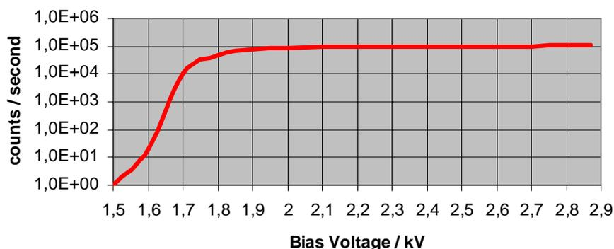
Fig.5: Typical Count-Rate/Bias Voltage Curve (Single Photo Electron Plateau) when constant light level is applied
