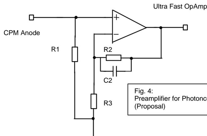
Fig. 4: Preamplifier for Photoncounting circuit (Proposal)
