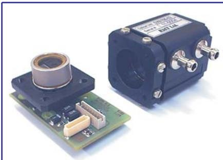
*Fig. 3.3. DX6106 Optical Unit with optopair detached*
