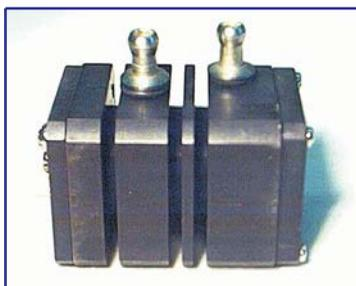
*Fig. 3.4. DX6106.C2 gas sampling cell*
