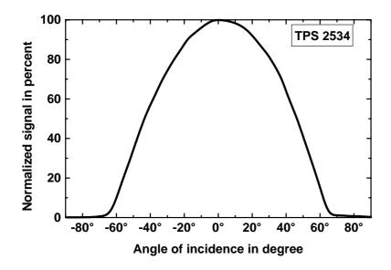
The graph shows the thermopile response as a function of the radiation incidence angle -90...+90°. Defining the field of view as the angle range, where the relative signal drops to 50% of its maximum value, the value of 90° is derived.
