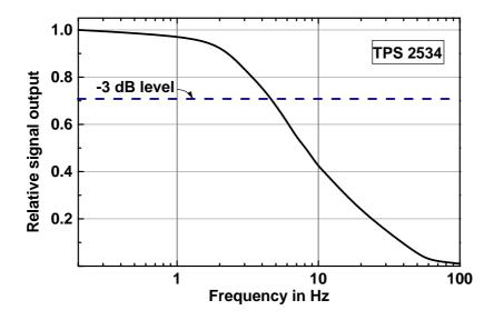
The figure shows the relative signal output as a function of the thermal signal chopping frequency. The -3 dB level at 71% relative output level defines the cutoff frequency  $f_{co}$  and thus the time constant  $\tau$  via  $\tau = 1/2\pi$   $f_{co}$ .
