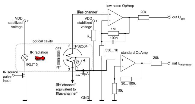
To amplify the thermopile signals, select a low noise operational amplifier. Recommended types are e.g. Intersil Harris ICL7650, Linear technology LT1112 (Dual) / LT1114 (Quad), or Analog Devices AD8551 / AD8552 / AD8571 / AD8572. Attention: If you do not employ a rail-to-rail amplifier, either a dual polarity power supply or a bandgap voltage is needed.
