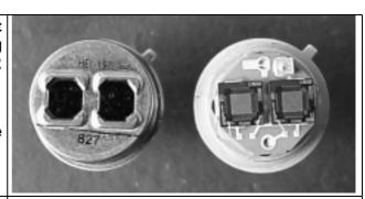
TPS 2534: 4 pin sensor housing of TO 5 size
