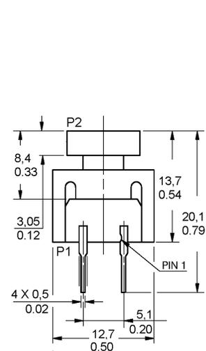
\*Recommended torque for sealing is 4 in-lb. Do not exceed 6 in-lb of torque. Use size 007 O-Ring. O-Ring counterbore dimensions are 0.04 ± .005 in D x 0.300 ± .003 in Dia.
