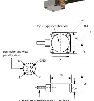
4 conductor shielded cable 1,8 m. long with 76 mm of jacket and shielding removed and wires braided and terminated with a 4-pin pos. connector
