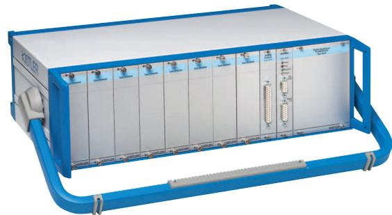
The base unit (Master) can be supplemented by one 19" additional unit (Slave), in which data communication continues to take place via the base unit. ("Combustion engines" sector).
