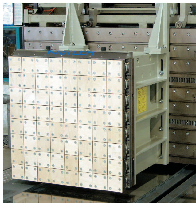
Fig. 4: Standard SmartCrash segment, prepared for EuroNCAP with plywood protection plates, without deformable element (honey-comb)
