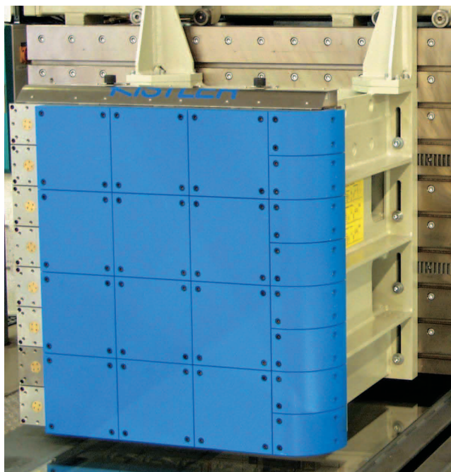
Fig. 5: Standard SmartCrash segment, prepared for RCAR/AZT with profiled aluminium corner elements R = 150 mm and aluminium front protection plates 250x250 mm
