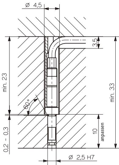
Fig. 2: Mounting with spacer sleeve Type 6464A3
