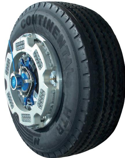
cell stores all important component parameters and prevents a misidentification of the load cell data. When the measuring system is powered up, the data of the components currently in use is imported into the connected System 2000 on-board electronics.
