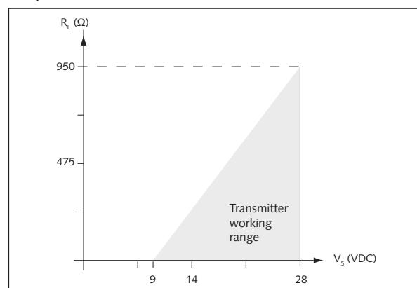
**Load Chart for 4 ... 20 mA (loop powered current output)**
