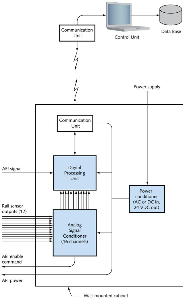
Fig. 1: Block diagram of Rail WIM system
