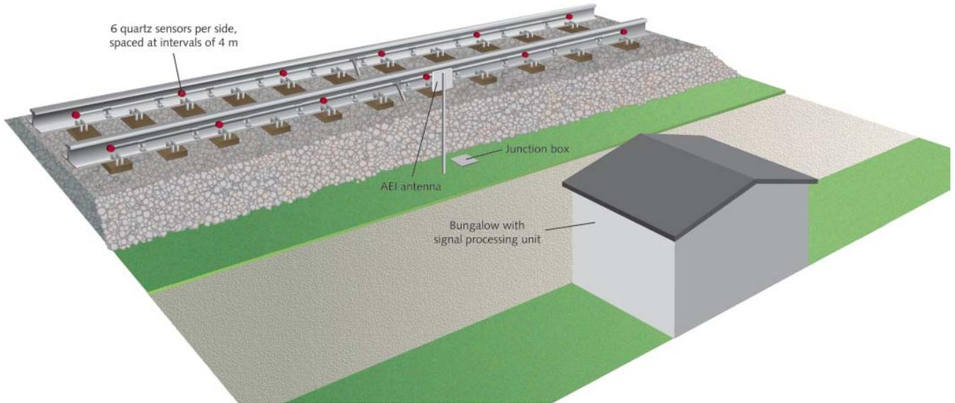
Fig. 3: Rail WIM system – standard layout
