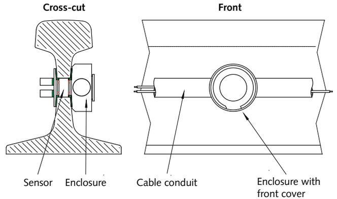
Fig. 2: Sensor assembly with conduit
