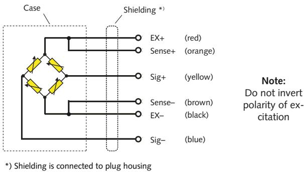
Fig. 1: Schematic diagram of one axis (the sensor has three axes)
