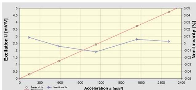
Fig. 2: Typical pendulum calibration (z-axis)
