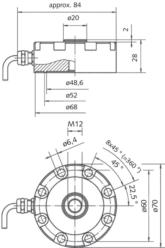
Fig. 1 : Dimensions strain gage load cell Type 4578A...
