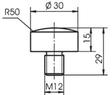
Fig. 2: Force distributing cap Type 4578AZ01
