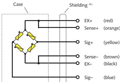
\*) Shielding is connected to plug housing
