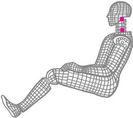
Fig. 1: Dummy application, location upper & lower neck
